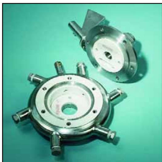
Easily opened Micronizer shows aluminum oxide, wear-resistant liners.
