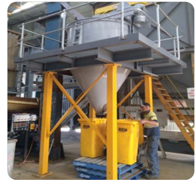
Whirlwind installation requires NO process dust collector
