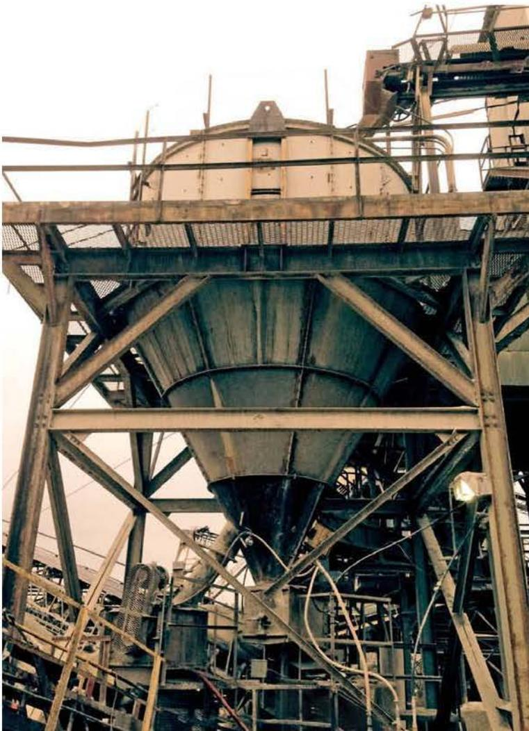
The Sturtevant 16-ft. Whirlwind air classifier produces aglime and concrete sand.
