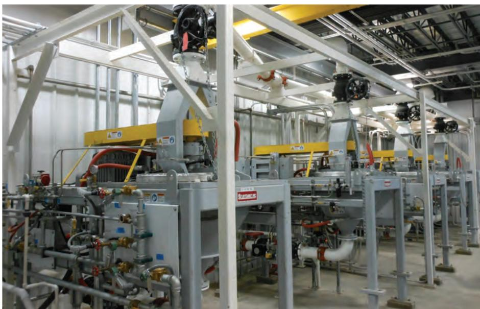
**FIGURE 4.** In recent years, pin mills, such as this one milling trona, have become competitive with air-swept classifying mills on performance, but also can yield reduced capital, energy and operating costs
