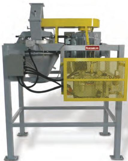
**FIGURE 2.** Pin mills can be configured in many ways to suit the needs of the application (for instance, using vertical or horizontal shaft, pneumatic or gravity-feed options, varying materials of construction and pin configurations) and more
