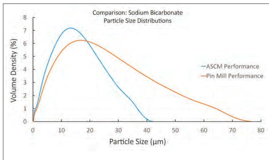
**FIGURE 3.** Shown here is a comparison of the particle-size distribution for a pin mill versus an airclassifying mill handling sodium bicarbonate. As shown, the pin mill was not able to achieve the same maximum fineness as the final product produced by the air-swept classifying mill
